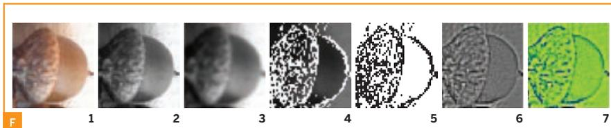
Excel. Image 2 is a grayscale version of 1. In 3, I blurred the image by averaging each pixel's value with that of its neighbors. In 4, I highlighted high-contrast areas by comparing each pixel with its neighbors. Image 5 shows only the high-contrast areas. In 6, the contrast values that I used to make 5 were converted into continuous grayscale (6), and in image 7, this grayscale image was converted to color (in ImageJ, not Excel) using a lookup table.
